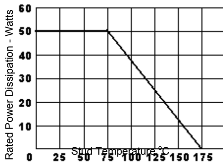
FIGURE 1 Power Derating Curve
